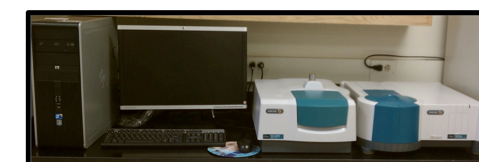
Figure 4. Cary Bio 50 UV-VIS Spectrophotometer (Varian, Inc.)
