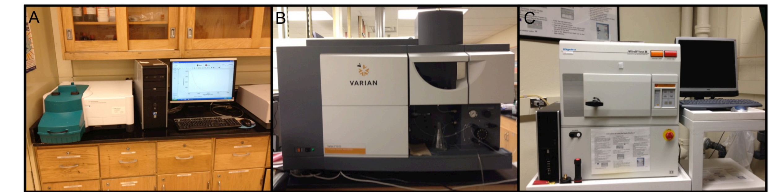
Figure 4. (A) Cary Eclipse fluorescence spectrophotometer (Agilent Technologies). (B) 710-ES ICP-OES spectrometer (Varian, Inc.). (C) Miniflex II X-ray diffractometer (Rigaku Corp.).
